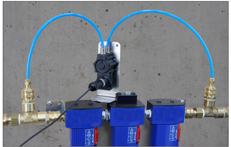
Typical application of the differential pressure sensor: connection with two PE hoses before and after the filter elements.
