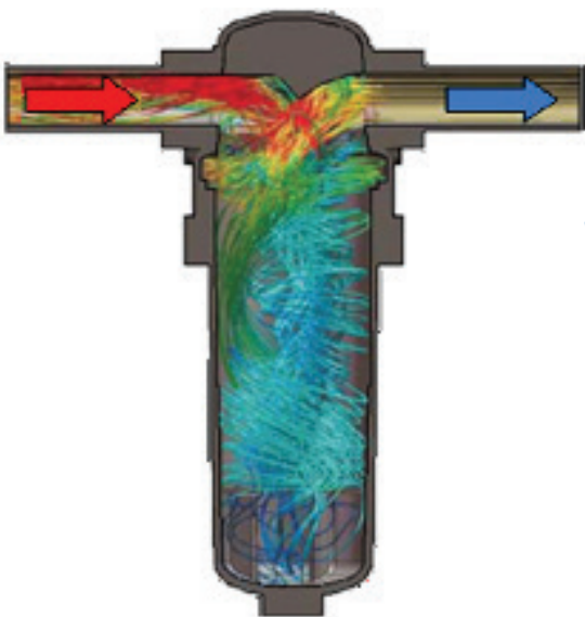
Air flow in a SPC cyclonic separator
