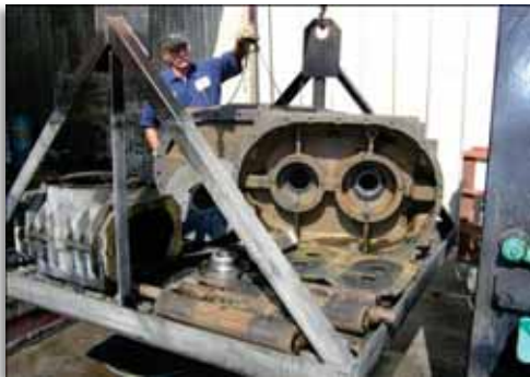
Parts Cleaned to White Metal
