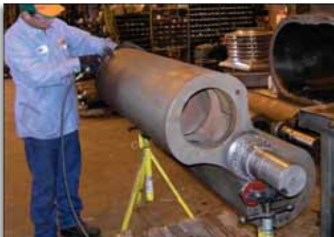
Impeller Hand Polished
